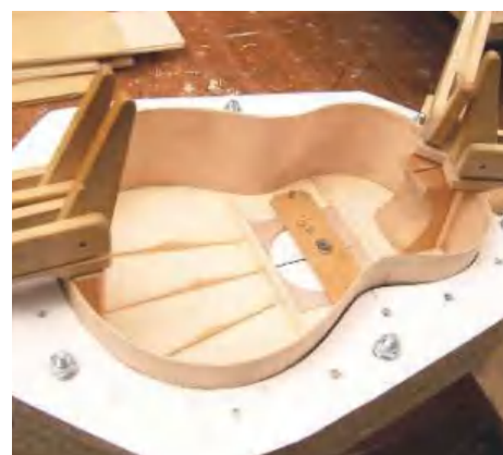
STEP 17. Fitting the front of the ukulele
